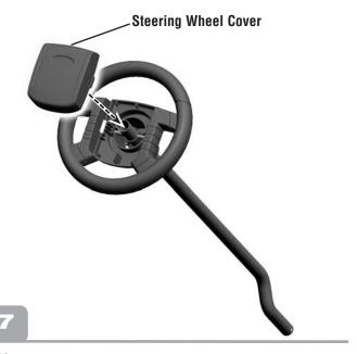
• "Snap" the steering wheel cover onto the steering wheel. *Hint:* If the steering wheel cover does not "snap" onto the steering wheel, you have not properly assembled the steering column to the steering wheel. Remove the pin and the steering column from the steering wheel and refer back to Assembly steps 5 and 6.
